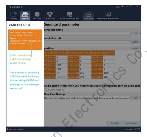
Resolution correct, cards number at least 1, means communication between sender and receiver is good.
