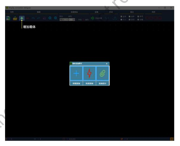
If the led screen contains various types of cabinets (different cabinet size, different driver ic or module design), please choose the first way (general add) and then click view www.sysolution.net
